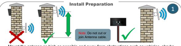
Mount the antenna as high as possible and away from obstructions such as vehicles, shrubs and trees to maximize signal strength.
